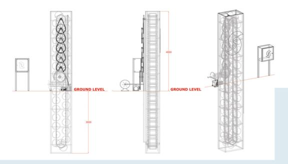
ROSCH THRUST KINETIC GENERATOR consists of one well (6m depth) filled with water wherein the plastic chambers (floats) are submerged and connected to a transporting system.
